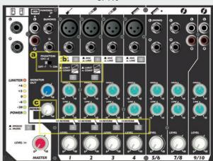
Phantom Power: Provides 15V DC phantom power for condenser mics on 4 mic channels.
